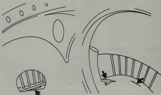
Cracked area along spot weld line on inner duct.
